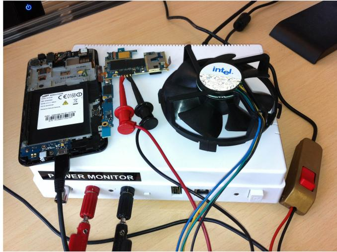
Fig. 2. Measurement setup showing the power gauge (below), the disassembled Samsung Galaxy S2 (left), the fan (right), and its switch, used to control the temperature of the testbed.
